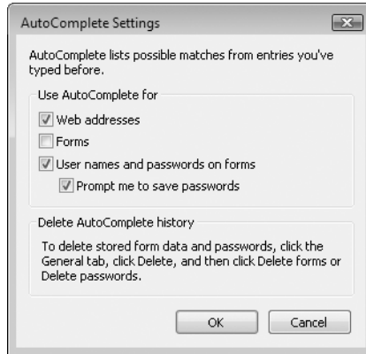
Figure 6-12 You can turn various AutoComplete options on or off individually.
