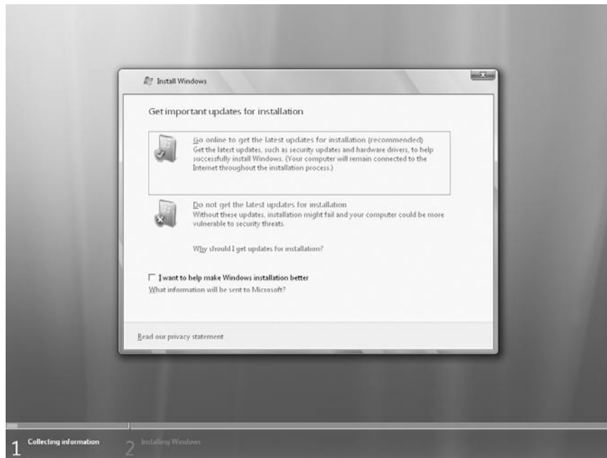
Figure 2-5 For an upgrade installation, you'll avoid headaches if you take advantage of the option to download security updates and new drivers as part of setup.
