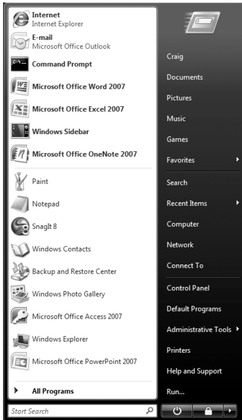
Figure 3-16 The default Start menu provides a place to “pin” your most frequently needed programs, displays recently used programs below that, and offers access to crucial system folders on the right.
