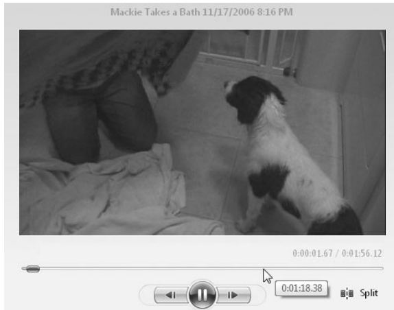
Figure 18-9 Aim the mouse pointer at the Seek bar to see this ScreenTip, which shows the time marker for that point on the bar. Click to jump to that point.
