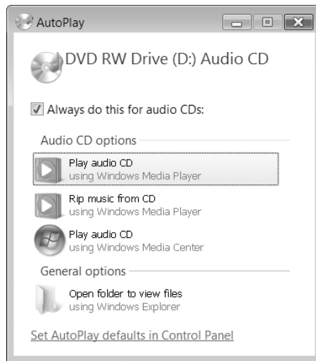
Figure 3-35 The AutoPlay dialog box that appears when you first insert an optical disc of a given type lets you tell Windows how to process the disc—either this time or every time.
