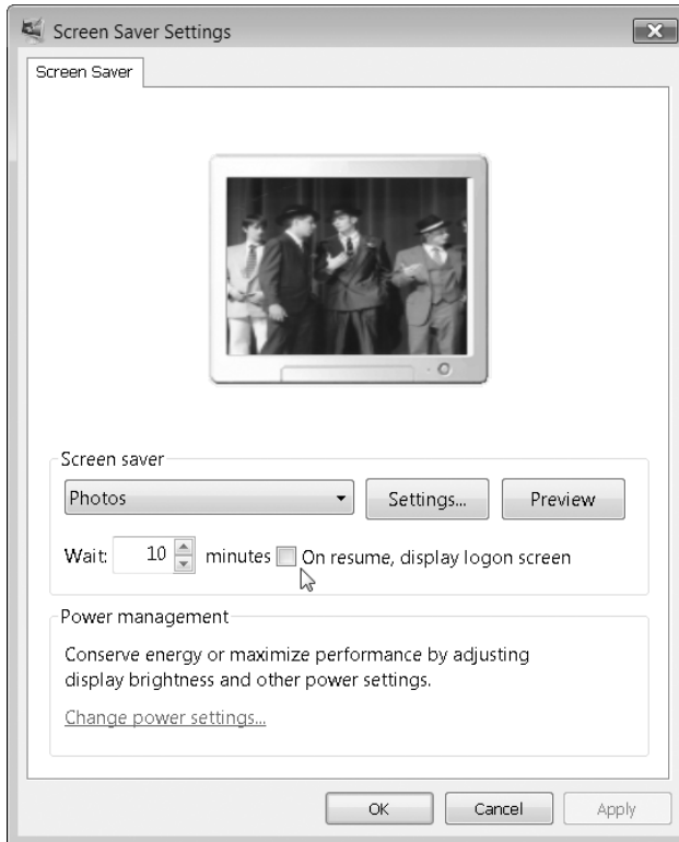
Figure 3-9 Clearing the On Resume, Display Logon Screen in the Screen Saver Settings dialog box can save you the trouble of logging in every time you return to your desk.
