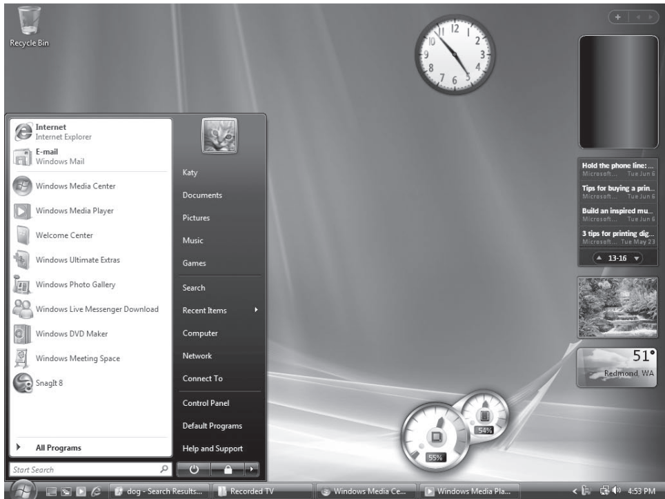
Figure 1-2 The All Programs menu slides smoothly instead of flying out to the right, and Sidebar gadgets add information and entertainment to the desktop.
