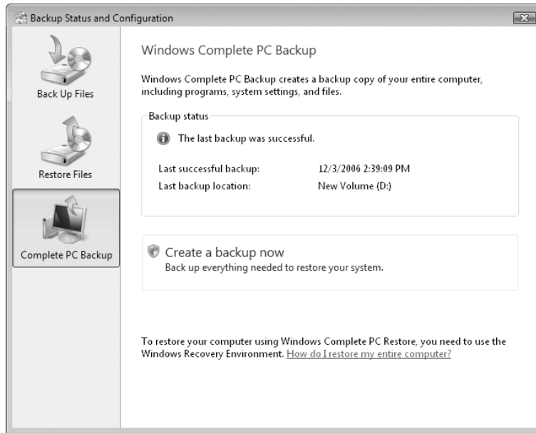
Figure 2-19 The Complete PC Backup feature (available only in Business, Ultimate, and Enterprise editions) allows you to create a snapshot of a working system that can be restored in minutes.
