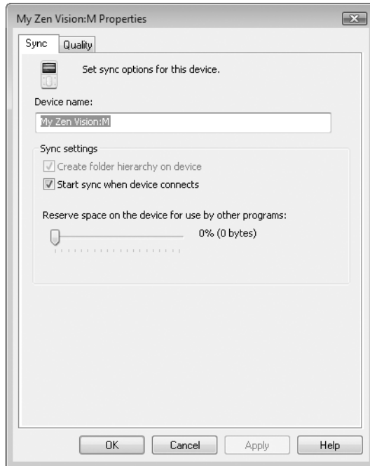
Figure 15-10 Some synchronization options are unavailable when the hardware doesn't support changes to those features.
