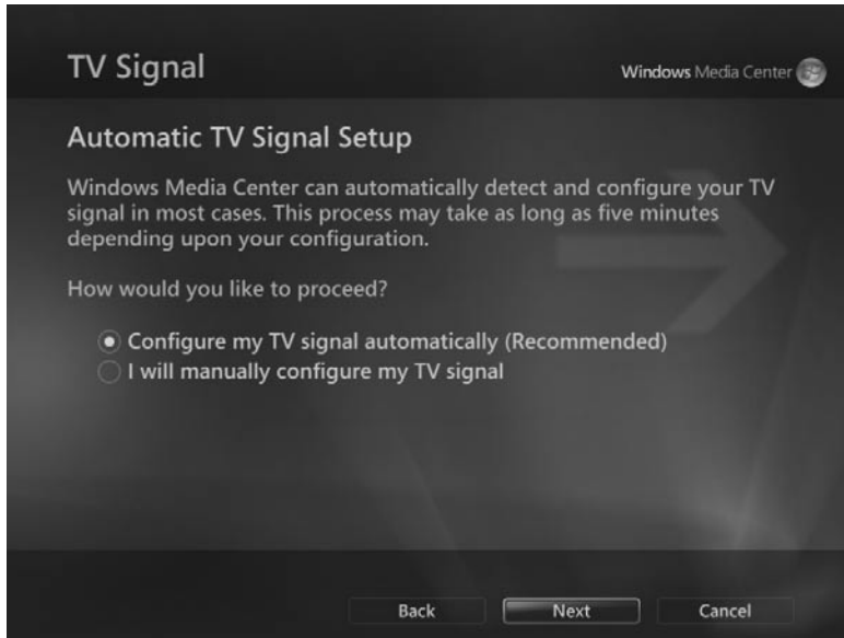
Figure 19-5 Always try to use the automatic setup first. If setup is unsuccessful, you'll be offered the option to start over and choose manual settings.
