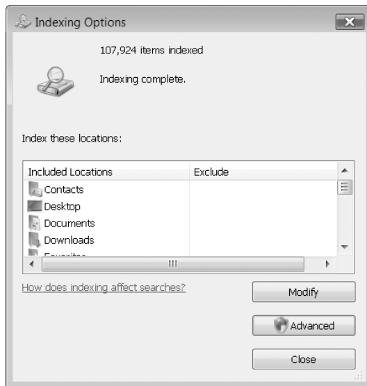
Figure 7-27 The Indexing Options dialog box shows you how many items have been indexed and whether the index is up to date.
