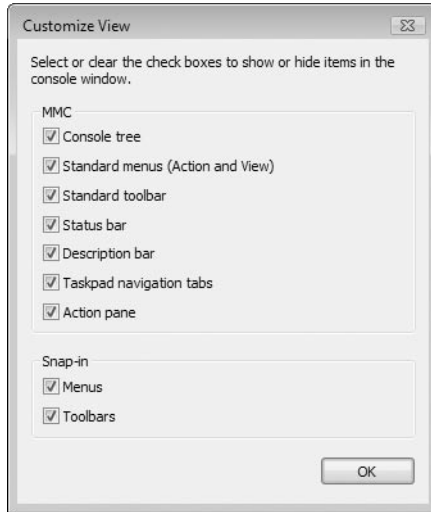
Figure C-3 You can use the Customize View dialog box to control various elements of the MMC console, which are identified in Figure C-1.
