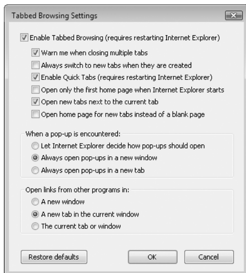
Figure 6-5 Use any of the options shown here to change the behavior of tabbed browsing—or disable it completely.
